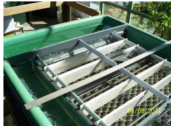
Figure 3 a and b: Experimental setup of the past project (UFT 2013) with Leiblein upflow honeycomb lamella modules
