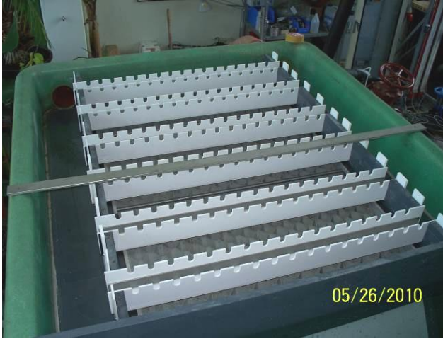
Figure 4: Final arrangement of overflow flumes (the shown camera date is wrong, the pictures are from June 2011)
